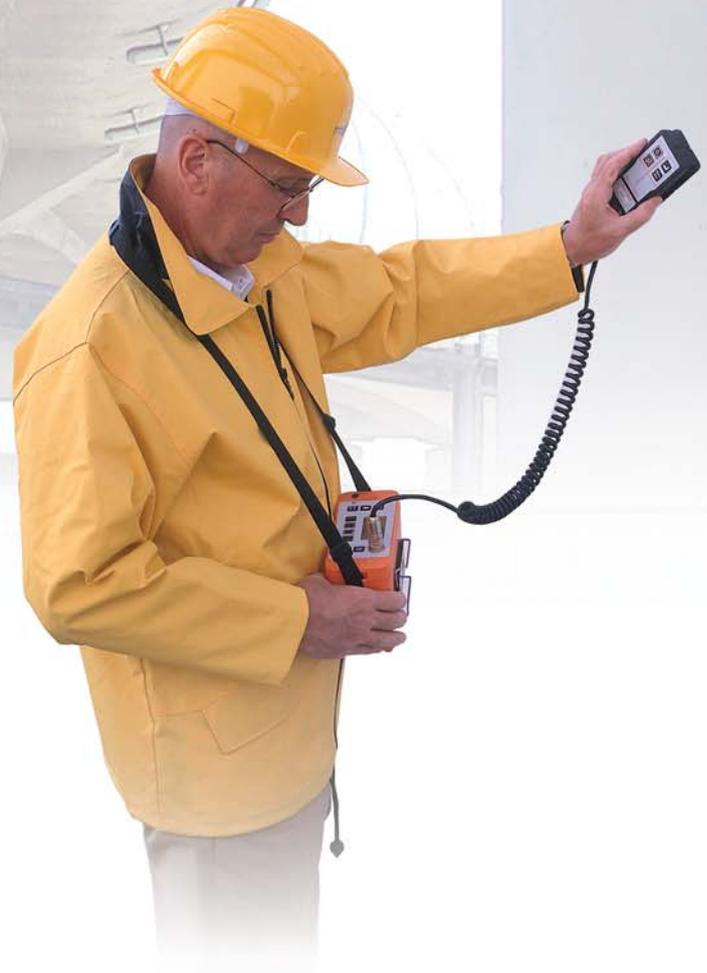
**BARTRACKER** in use on concrete column reinforced with steel bars.
