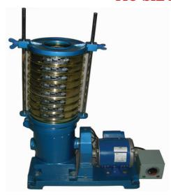
"TIC" **Gyratory** type sieve shaker is driven by 1/2 HP Crompton Motor through a reduction gear. Suitable to carry 8" dia upto 7 sieves. When clamped the sieve table inclines from the vertical axis and the direction of inclination changes progressively in the clockwise direction. The shaker also gives an up and downward movement at a frequency of approx. 270rpm.
