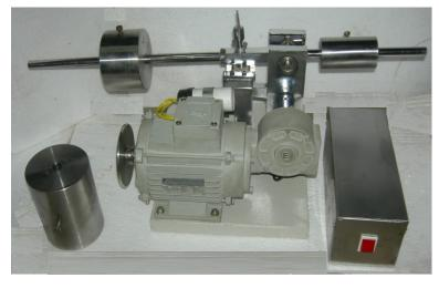
To examine the sensitivity of solids and pastes to sliding (frictional) contact. Designed and manufactured to permit testing to the UN Transport of Dangerous Goods recommendations, Manual of Tests and Criteria and to the European Classification, Packaging and Labelling of Dangerous Substances in the European Union, testing methods.
