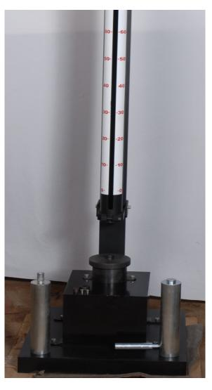
To study the impact sensitivity of solids and liquids. Designed and manufactured to permit testing to the UN Transport of Dangerous Goods recommendations, Manual of Tests and Criteria and to the European Classification, Packaging and Labelling of Dangerous Substances in the European Union, testing methods.
