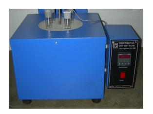
To study the chemical sensitivity and stability of solids and liquids explosive in nature. Designed and manufactured to permit testing to UN/NATO and other similar standards for Dangerous Goods and explosives. The instrument continously monitors and records the pressure change in the tube containing the sample at set temperature.
