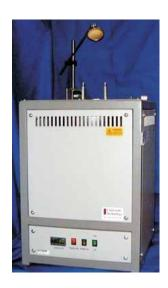
For determining the temperature at which a gas or vapour will auto ignite. Equipment can be supplied in accordance with ASTM, DIN, IEC or to the European Classification, Packaging and Labelling in the European Union test standard. It comes complete with high speed data acquisition system.
